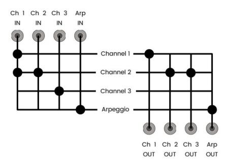
Now let's look at how channel 2 operates here: The pitch that is read at channel 1's IN jack is being **added** to that of Channel 2's IN jack. The resulting input pitch is then quantized through Channel 2. The resulting output pitch of Channel 2 is output not only on Channel 2's OUT jack but also at Channel 3's OUT jack.
