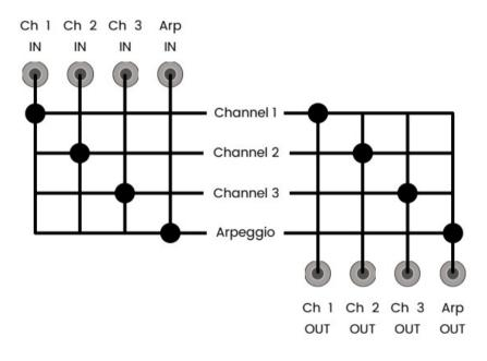
The pitch input of the IN jack of channel 1 is being sent to channel 1, quantized there and output at the OUT jack of channel 1. Not very surprising.
