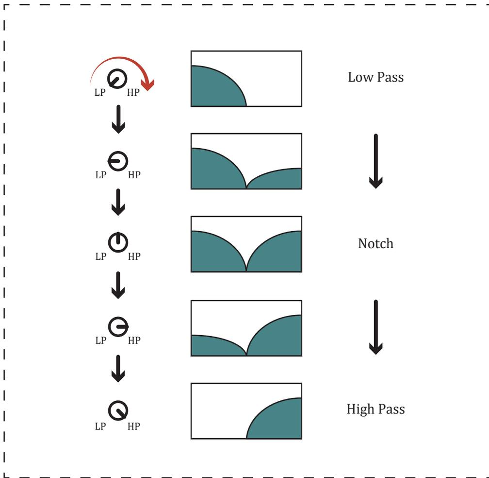
FIG.3: Filter type change by "LP HP" knob setting
