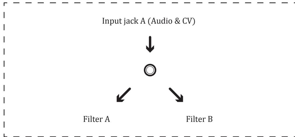
FIG.6: When only input A is plugged in (Normalized)
