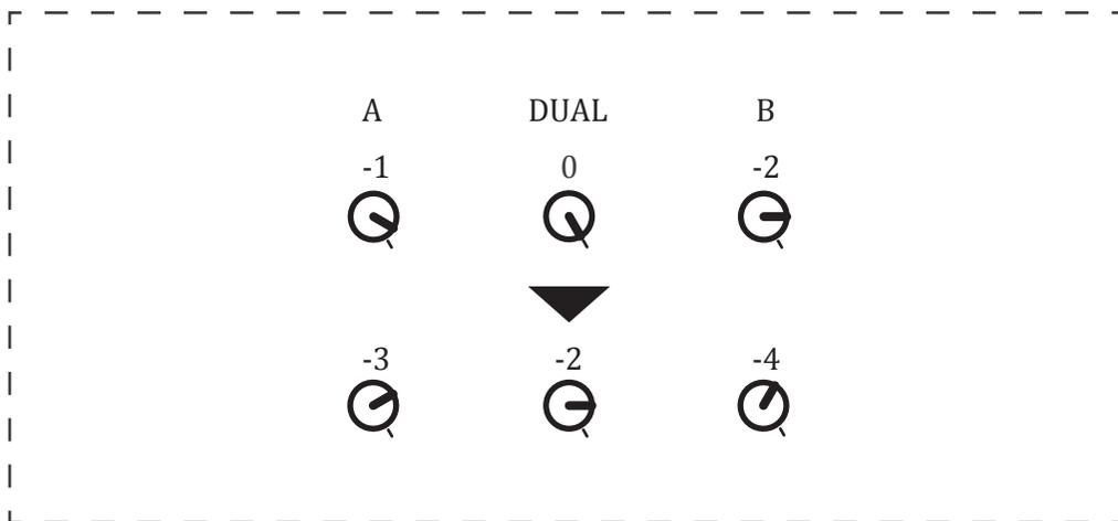
FIG.5: Reaction of CUTOFF A, B in conjunction with the operation of DUAL CUTOFF
