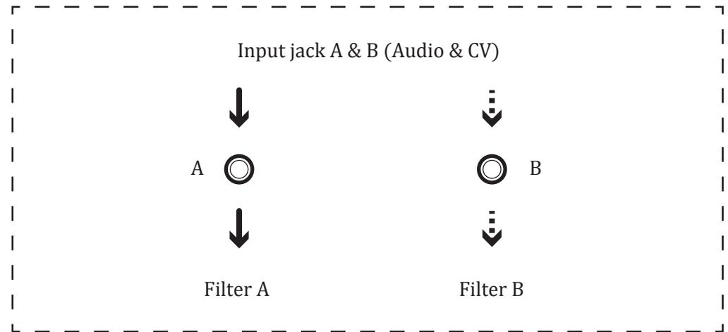
FIG.7: When inputs A and B are plugged in (not Normalized)
