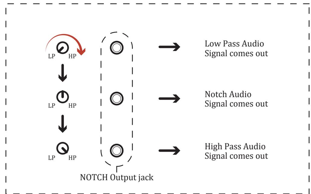
FIG.4: Changing audio output signal from "Notch" jack by "LP HP" knob setting
